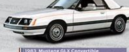
1983 Mustang GLX Convertible ENGINE: 231 cubic inch (3.8L) V6 HP: 112 BODY: Coupe, convertible and hatchback.
