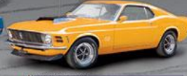
1970 Boss 429 ENGINE: 429 cubic inch V8 HP: 375 BODY: Coupe, convertible and fastback. GT was removed from the lineup until 1992.
