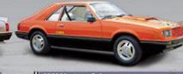
1981 Mustang Cobra ENGINE: 4.2 liter V8 HP: 120 BODY: Coupe and hatchback. First year that hatchbacks outsold coupes. 2
