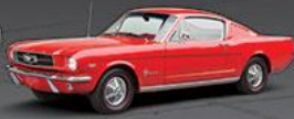
1965 Mustang 2+2 Fastback ENGINE: 289 cubic inch V8 engine HP: 271 BODY: Coupe and convertible. Fastback was added.
