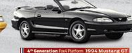
4th Generation Fox Platform 1994 Mustang GT ENGINE: 301 cubic inch (5.0L) V8 HP: 240 BODY: Coupe, convertible and hatchback.
