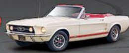
1967 Mustang GTA ENGINE: 390 cubic inch V8 HP: 320 BODY: Coupe and convertible. Only year for the GTA.
