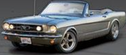
1st Generation Falcon Platform 1965 Mustang ENGINE: 289 cubic inch V8 engine HP: 271 BODY: Coupe and convertible
