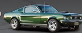
1968 Mustang 2+2 Fastback Cobra Jet ENGINE: 428 cubic inch V8 HP: 335 BODY: Coupe, convertible and fastback.
