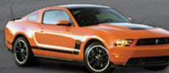
2012 Mustang Boss 302 Coupe ENGINE: 302 cubic inch (5.0L) V8 HP: 444 BODY: Coupe and convertible. Boss name restored.
