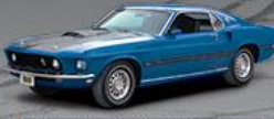
1969 Mustang Mach 1 Cobra Jet ENGINE: 428 cubic inch V8 engine HP: 335 BODY: Coupe, convertible and fastback. Mach 1
