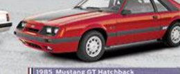
1985 Mustang GT Hatchback ENGINE: 301 cubic inch (5.0L) V8 HP: 210 BODY: Coupe, convertible and hatchback.
