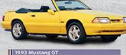
1993 Mustang GT ENGINE: 301 cubic inch (5.0L) V8 HP: 205 BODY: Coupe, convertible and hatchback.
